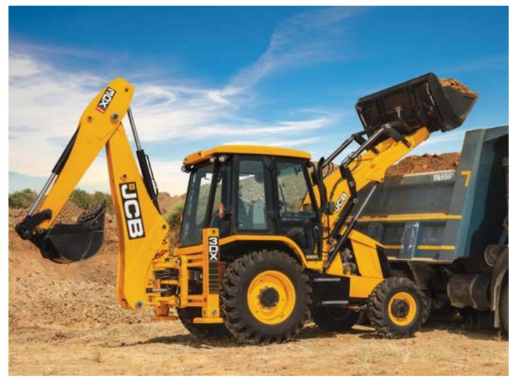
The 3DX PRO has a high flow piston pump which improves controllability and causes the engine speed to be reduced, saving fuel whilst maintaining performance.
